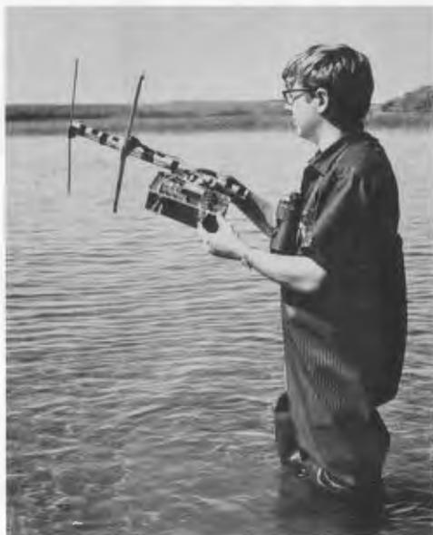
Fig. 4 Hand-held portable receiving system used for monitoring the activity of radio-tagged birds at distances of three miles. This instrument is sensitive enough to enable the investigator to locate tagged birds in the dark when they are roosting 70 feet up in trees.
