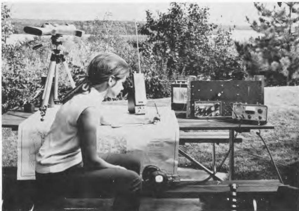
*Fig. 5 Base station located on hill near territory of one pair of birds being studied. Visual observations were made at distances of five miles with spotting scope and base and field personnel worked together using citizen band radios and tracking receivers located throughout the study area. Working range from base was approximately 22 miles.*
