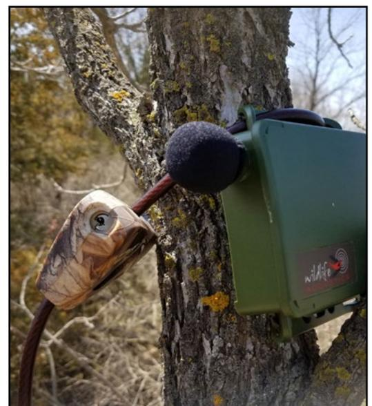
Song meter deployed with locking cable
